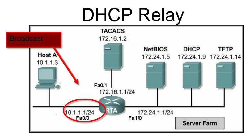
To configure RTA Fa0/0 (the interface that receives the Host A broadcasts) to relay DHCP broadcasts to the DHCP server, use the following commands:
